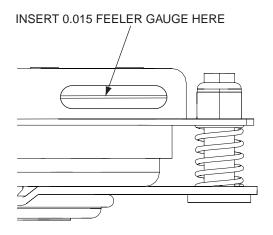
Figure 6-4. Clutch Air Gap Adjustment
